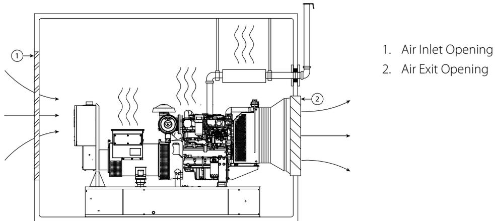
Figure 4.1 – Typical installation showing generator set ventilation
