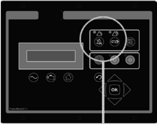
If either of these indication lamps are flashing or solid there is a warning or shutdown
