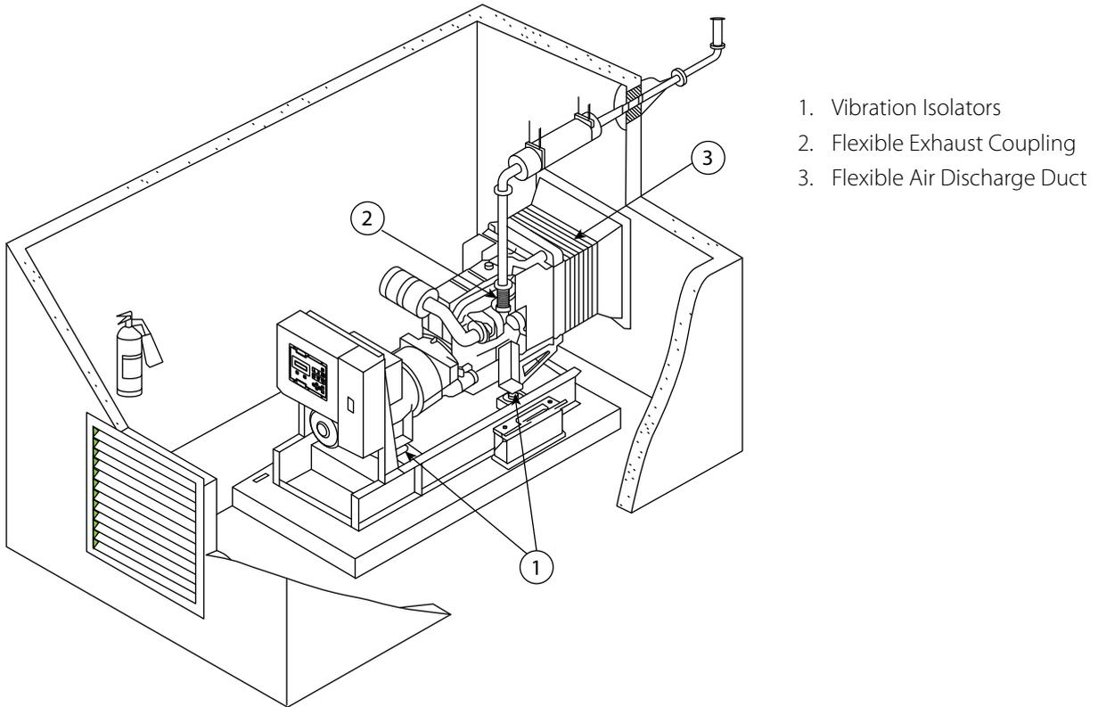
Figure 4.11 – Typical installation highlighting vibration reduction techniques
