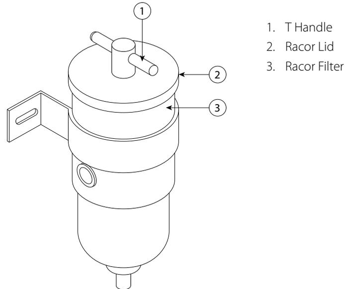
Figure 6.2 – Example of a Racor
