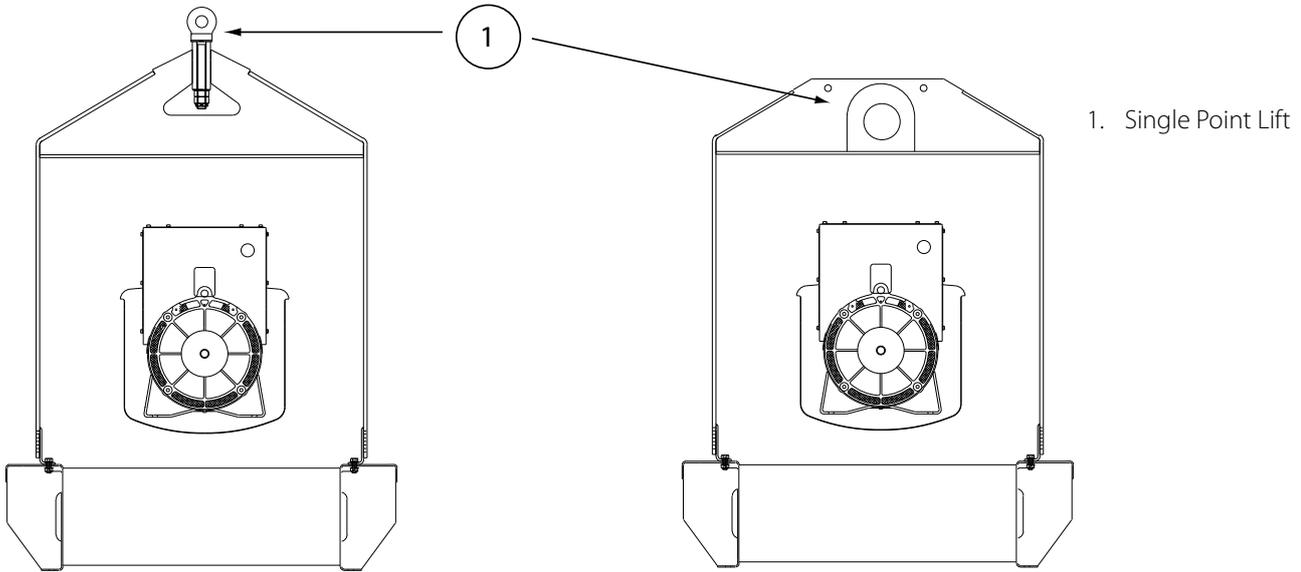
Figure 4.6 – Single Point lift
