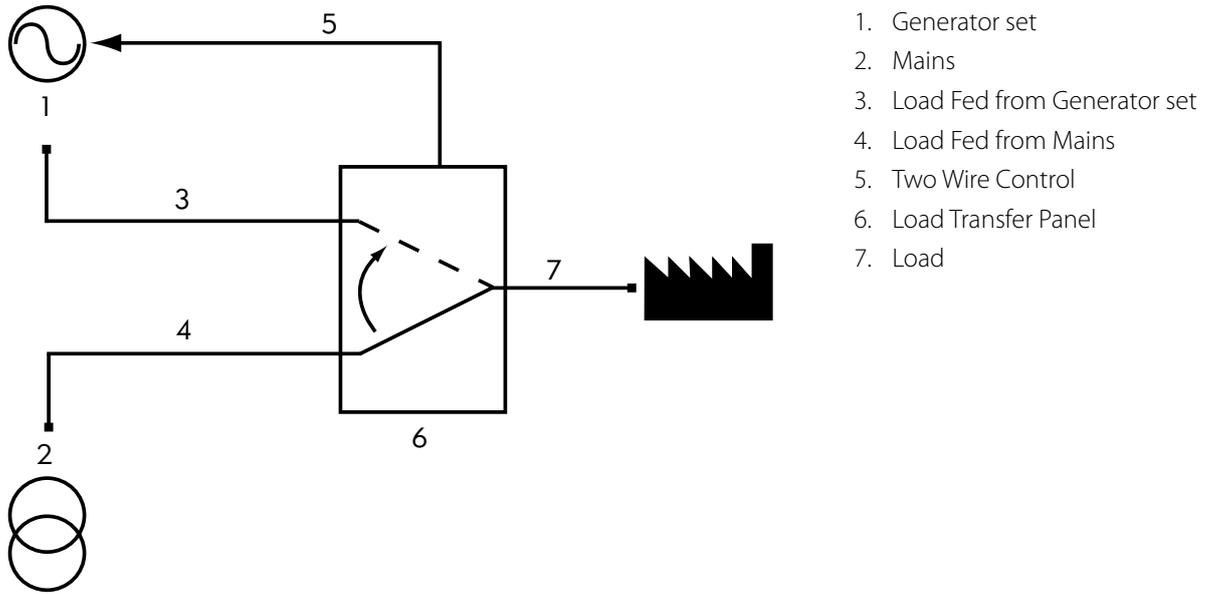
Figure 7.1 – Function of a Load Transfer Panel
