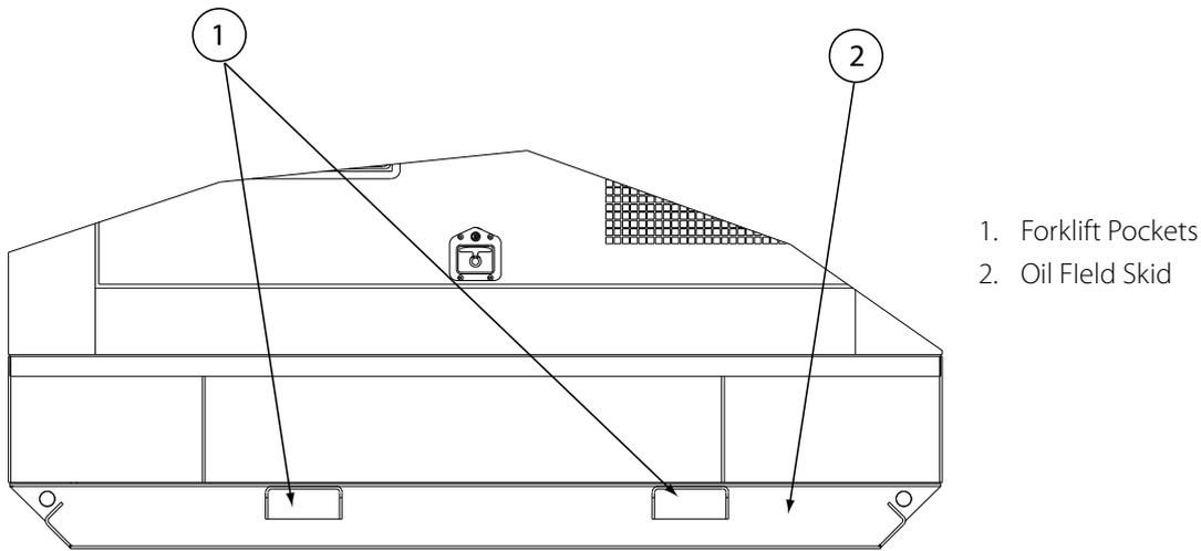
Figure 4.5 – Typical generator set with Oil Field Skid base option
