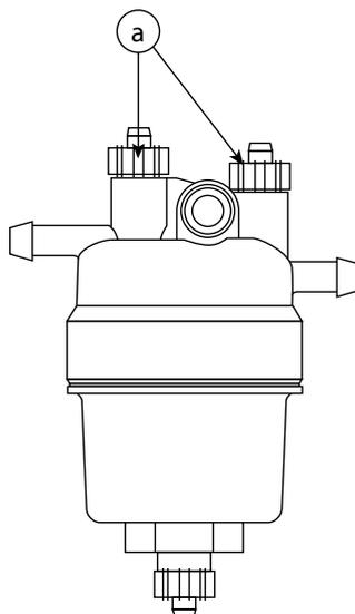
Figure 6.1 – Example of pre-filter / water separator
