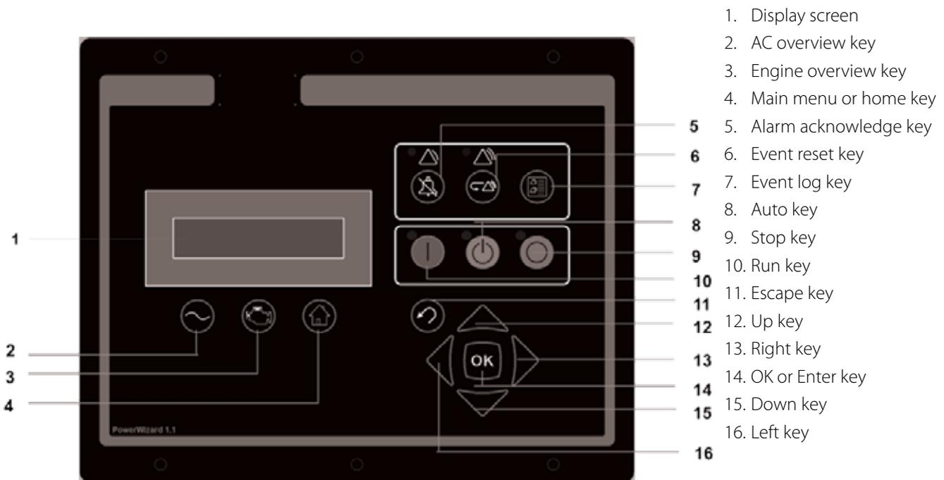
Figure 5.2 – PowerWizard Control Module Description
