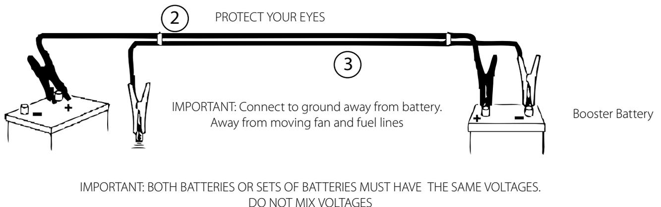
Figure 6.4 - Starting using jump start cables
