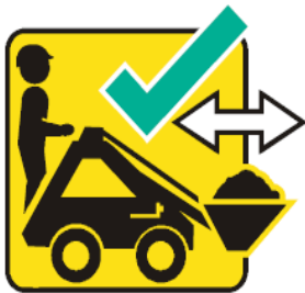
5. TRANSPORT MATERIAL WITH BUCKET DOWN AND LEVEL
