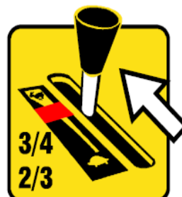
15. OPTIMUM OPERATION OF THIS MACHINE IS ACHIEVED AT 2/3 TO 3/4 THROTTLE
