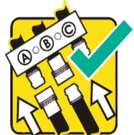
4. ENSURE HYDRAULIC HOSES ARE CLEAN AND ATTACHED
