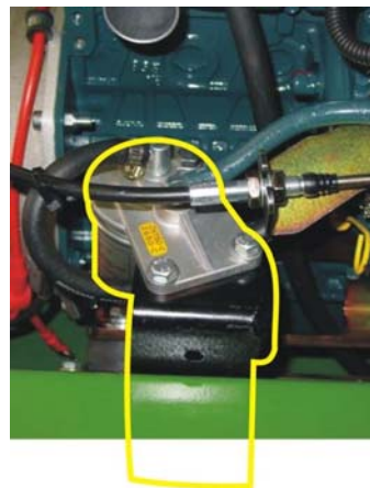
Photo showing current model fuel filter and mounting bracket from Mid 2008 .
