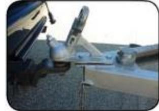
4. \*NOTE\* the jockey wheel ONLY sits vertical when trailer is NOT connected to the vehicle or whilst being lowered onto the vehicle\*. Once trailer is secured onto the ball, you will need to pull the handle next to the jockey wheel out to enable it to rotate and sit in a horizontal position. You must ensure that the pin on the handle of the jockey wheel locks into place to hold the jockey wheel horizontally. The jockey wheel MUST be horizontal before towing commences.
