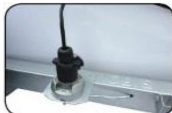
7. You will see a small latch sitting behind the coupling on the trailer, this is the reversing latch. It will be in the OFF position. In this position, the trailer brakes will NOT work. The latch WILL need to be in this position when reversing. Flick the latch into the opposite position to enable the brakes to work.
