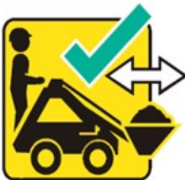
5. TRANSPORT MATERIAL WITH BUCKET DOWN AND LEVEL
