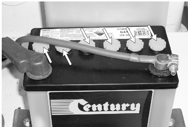
Figure 7.7 - Battery Fluid Level
