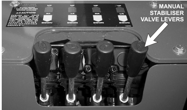
Figure 6.7 - Stabiliser Controls (Manual)
