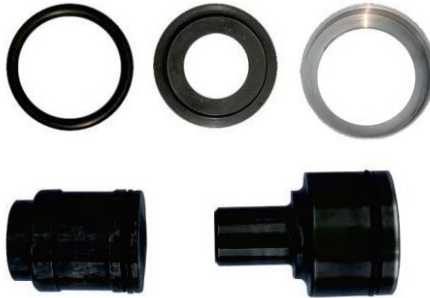
Figure 5: damper assembly, top & bottom hammer
