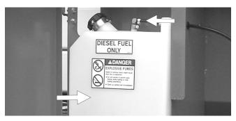
Figure 7.3 - Fuel Leaks at Tank
