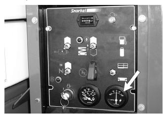
Figure 4.2 - Ammeter Gauge
