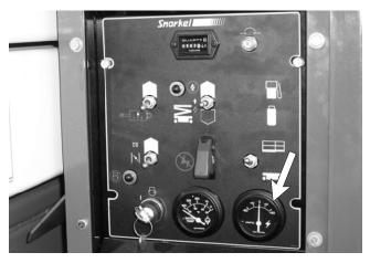
Figure 7.23 - Ammeter Gauge
