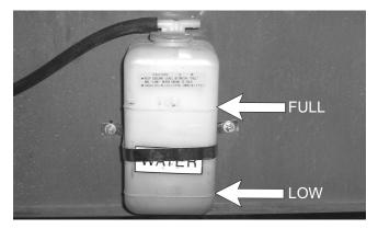
Figure 7.6 - Engine Coolant Level
