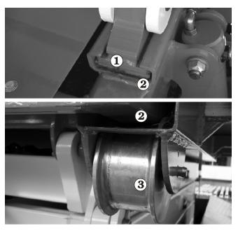
Figure 7.22 - Guides Rollers and Slides
