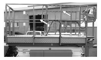
Figure 7.20 - Guardrails
