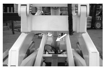
Figure 7.15 - Check Hydraulic Cylinders
