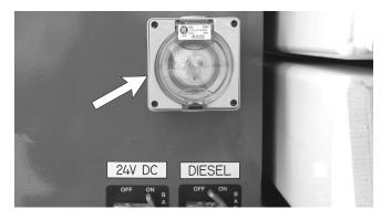
Figure 11.9 - Mains Power Connection For Charger
