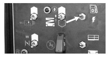
Figure 11.2 - Diesel/Electric Selection Switch
