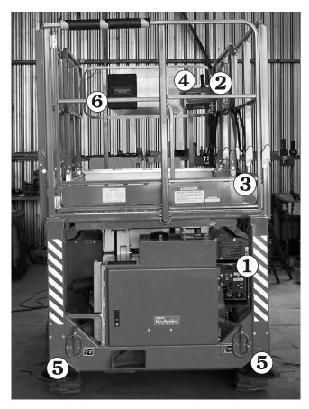
Figure 10.1 - Correct Stowed Position
