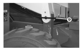
Figure 9.6.2 - Manual Bleed Down Control -Units Fitted With 24V DC Option
