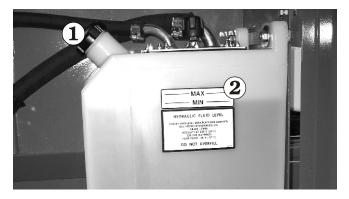
Figure 7.13 - Hydraulic Oil Tank
