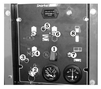
Figure 6.3 Ground Control Box Controls
