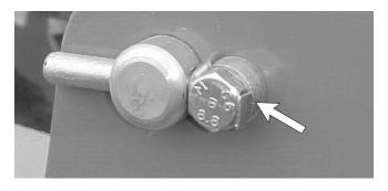
Figure 7.17 - Critical Pin Retainer Bolts
