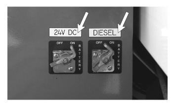
Figure 11.5 - Master Battery Isolator Switches
