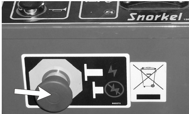
Figure 2.1 - Platform Control Box Emergency Stop Switch
