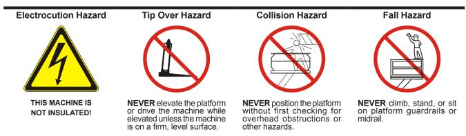
**USE OF THE AERIAL WORK PLATFORM:** This aerial work platform is intended to lift persons, their tools and materials used for the job. It is designed for repair, assembly, stockpicking jobs, etc., and assignments at workplaces above head height (ceilings, cranes, roof structures, buildings, shelving, etc.). All other uses of the aerial work platform are prohibited and the rules below must be adhered to!
