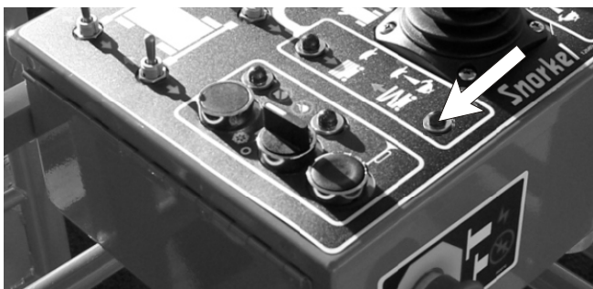
Figure 2.4 - Platform Overload Light
