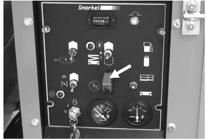
Figure 2.2 - Ground Control Box Emergency Stop Switch
