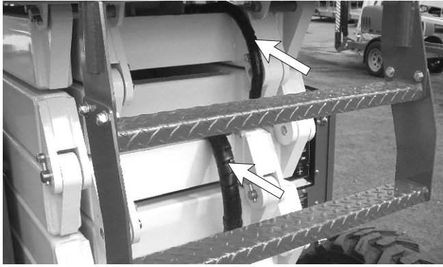
Figure 7.11 - Wiring Harness in the Scissor Stack
