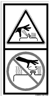
Fig. 19: Hydraulic oil tank under pressure
