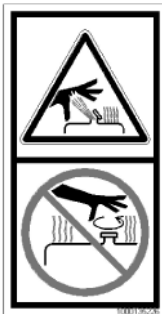
Fig. 19: Hydraulic oil tank under pressure
