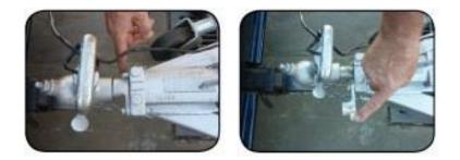
**<u>8.</u>** The handbrake lever will be in the ON position. Pleasure ensure the ratchet lever sits in the position as shown in the second picture below whilst towing the trailer.
