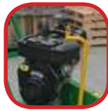
16hp(12kW) OHV V-twin Briggs & Stratton Vanguard
