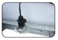
7. You will see a small latch sitting behind the coupling on the trailer, this is the reversing latch. It will be in the OFF position. In this position, the trailer brakes will NOT work. The latch WILL need to be in this position when reversing. Flick the latch into the opposite position to enable the brakes to work.
