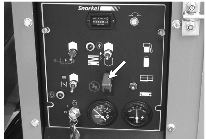
Figure 8.1 - Emergency Stop Switch at Ground Control Box
