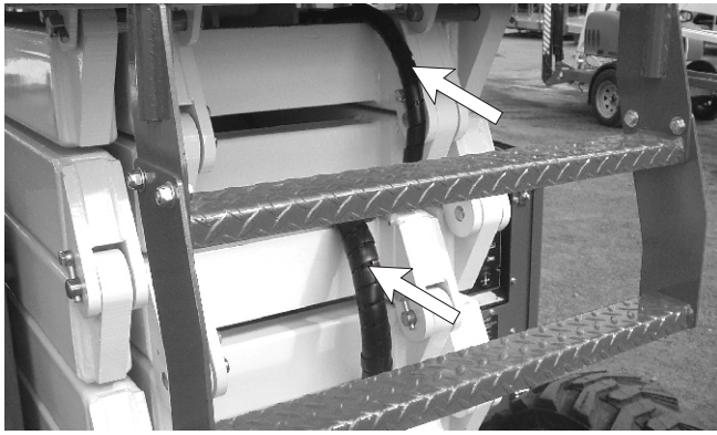
Figure 7.11 - Wiring Harness in the Scissor Stack
