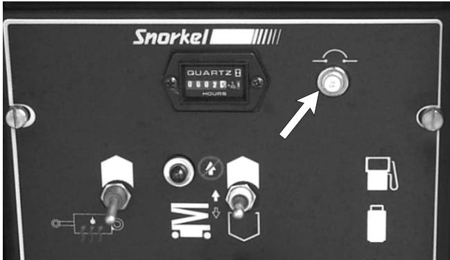
Figure 5.4 - Main Circuit Breaker
