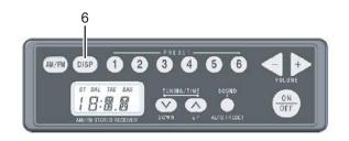
To switch the frequency display to the time display, press the "DISP" key in this condition. (To switch the time display to the frequency display, press the "DISP" key. After the display of station for 1.5 seconds, the display changes to frequency display.)
