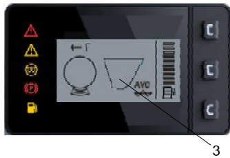
Fig. Working mode, Chip spreader (Off)
