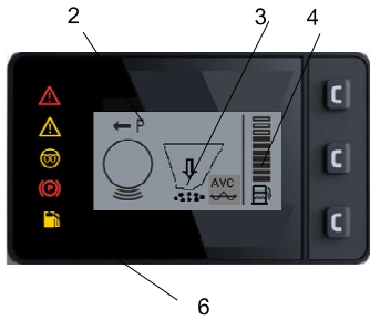
Fig. Working mode, Chip spreader (On)
