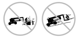
Limit travel speed according to the condition of the ground surface, congestion, slope, location of personnel, and any other factors which may cause collision.
