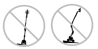
Do not raise or extend the boom unless the machine is on a firm, level surface.
