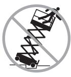
Do not operate the machine in strong or gusty winds. Do not increase the surface area of the platform or the load. Increasing the area exposed to the wind will decrease machine stability.
