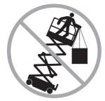
Do not place or attach fixed or overhanging loads to any part of this machine. Do not transport tools and materials unless they are evenly distributed and can be safely handled by person(s) in the platform.
