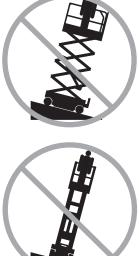
Do not raise the platform unless the machine is on a firm. level surface.
