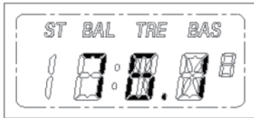
Frequency display (When stereo sound is not received, "ST" pict turns off)
