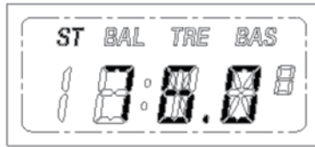
Frequency display (When stereo sound is received, "ST" pict turns on)
