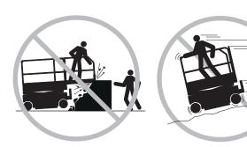
Limit travel speed according to the condition of the ground surface, congestion, slope, location of personnel, and any other factors which may cause collision.
