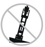
Do not depend on the tilt alarm as a level indicator. The tilt alarm sounds on the chassis only when the machine is on a slope.
