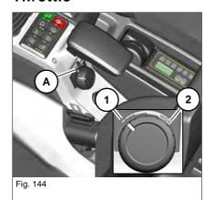
Engine speed can be set continuously with throttle A.
