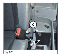
The cabin fuse box is located on the left of the operator seat.
