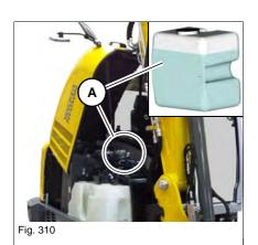
Reservoir filler inlet **A** is located on the right under the valve cover.
