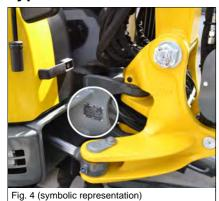
The vehicle type label is located at the right hand side of the vehicle, behind the swiveling console.
