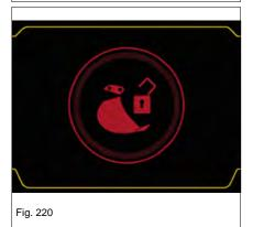
➡ The symbol Hydraulic quickhitch enabled appears and the buzzer sounds.
