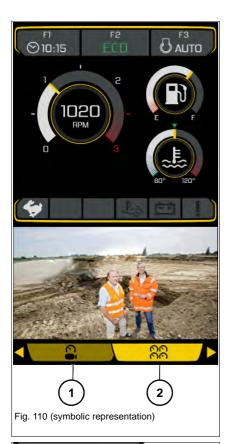
The reversing camera is located on top of the engine cover. It allows the operator to see the area behind the vehicle.
