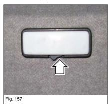
The mechanical switch above the left B-pillar must be in the position on the right so that the interior light can be switched on and off with the help of the switch panel.
