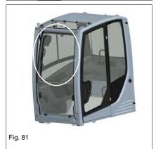
Opening the front window to a gap (ventilation position)
