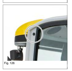
A 12 V connection is located at the rear right inside the cabin and on the right outside of the cabin.
