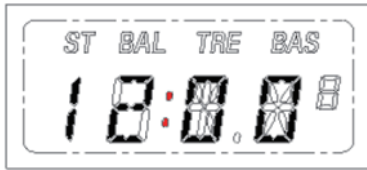
OFF (clock display) {Colon blinks (ON: 700 ms, OFF: 300 ms)}
