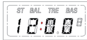
Clock display {Colon blinks (ON: 700 ms, OFF: 300 ms)}
