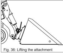
7. Raise the lift arm until the coupler begins to lift the attachment.
