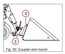
6. Move the machine forward until the coupler **(2)** is under the attachment's upper mount **(3)**.
