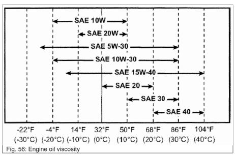
In particularly hot environments where ambient temperatures stay near and over 38°C (100°F), use SAE 15W-40 engine oil.
