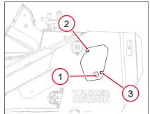
Fig. 58: Hydraulic oil sight glass and access plate
