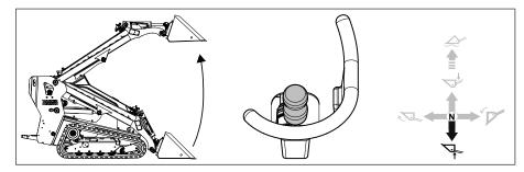
· Move the right joystick forward to lower the lift arm.
