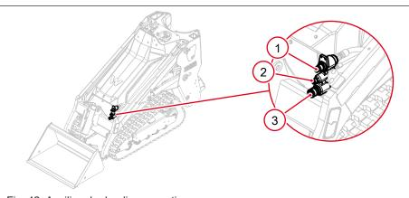
Fig. 42: Auxiliary hydraulic connections
