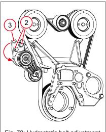
Fig. 78: Hydrostatic belt adjustment
