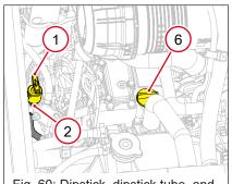
Fig. 60: Dipstick, dipstick tube, and oil cap
