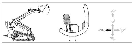
• Move the right joystick to the right to roll the attachment outward.
