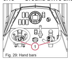
To have good control of the machine, move the levers smoothly, using the handrail (1) while operating.
