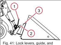
Fig. 41: Lock levers, guide, and mount
