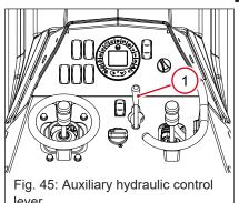
Push the auxiliary hydraulic control lever (1) forward for auxiliary hydraulic oil flow to the front male coupler. Hydraulic oil flow increases to the coupler as the lever is pushed forward.
