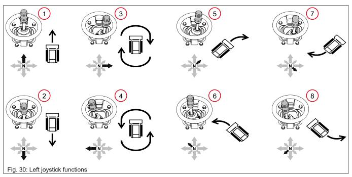
Refer to the illustration for the necessary joystick motions to move the machine as desired. Use the left joystick to move and turn the machine.
