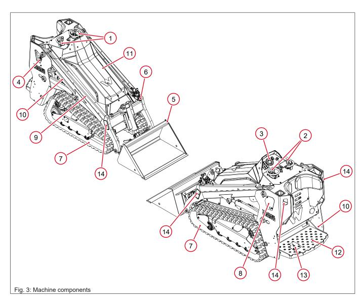
Ref. Component Ref. Component 1 Handrails 2 Controls 3 4 Diesel fuel fill Display Auxiliary hydraulic couplers 5 Attachment (options available) 6 7 Tracks 8 Hydraulic oil fill 9 Lift arm 10 Lift arm support device 11 Hood 12 Operator platform 13 14 Operator presence pedal Tie-down points
