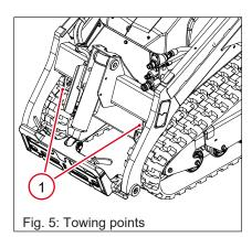
Do not tow this machine, except out of an immediate risk zone or to load onto a transport vehicle. Do not tow another machine with this machine. Only use the points on the frame (1) designated for towing.
