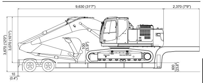
The dimensions and weight are 2.94m (9'-8") for the arm,  $0.8m^3 (1.05 \text{ cu} \cdot \text{yd})$  bucket, and 5.65m (18'-6") boom specification.
