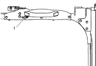
Hold and lift up the handles(2) on the upper and lower part of the front window (upper), and move the front window (upper) fully toward the back of the ceiling to automatically set it to the locked condition; however, check it is locked securely.
