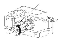
5. Remove equalizing filter (2).
