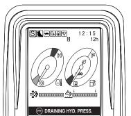
8. When the internal pressure release is failed, "FAIL DRAIN HYD. PRESS" is displayed on the multidisplay, and the buzzer sounds continuously. Perform Step 4 to 7, again.
