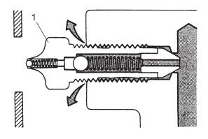
**Details of A Section (Grease Discharge)**
