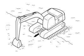
2. If the machine cannot travel due to highly tensed crawlers caused by clogged mud and gravel in the crawlers after traveling on the soft ground, lift each crawler off the ground by pushing the boom and arm against the ground and shake the mud or gravel off the crawler, and then get out of the soft ground. Gravel, or mud clogged in the crawler can be shaken off by lifting the crawler up and moving it forward and backward.
