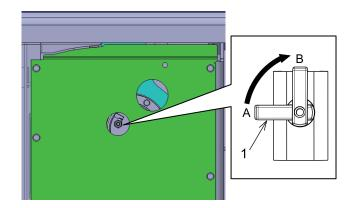
6. Set drain cock (1) to "CLOSED" position (B) when clean fuel comes out.
