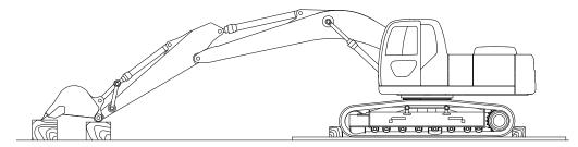
Store the machine in a dry indoor location. If you place the machine outside unavoidably, lay lumbers on a flat ground and cover the machine with a sheet. Especially, cover the muffler, hydraulic oil tank breather, fuel tank cap, and swing motor level gauge.
