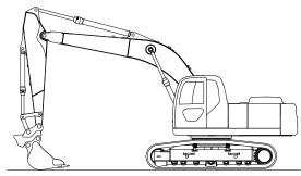
2. Push the "UNLOCK" side of the quick hitch operation switch to move movable hook (1) to release the front attachment. (See "QUICK HITCH OPERATION SWITCH" in Chapter 2.)
