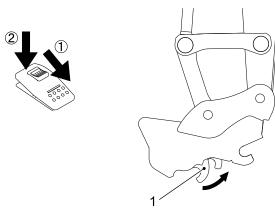
3. Move the attachment/equipment of the machine side to remove the front attachment.
