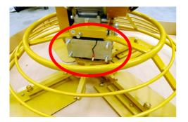
**STEP 3** – Fit handle end onto the studs, re-fit the Flat Washers, Spring Washers, Dome Nuts and tighten securely.
