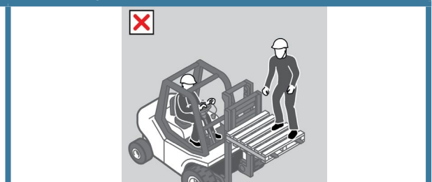
FIGURE 2 It is not safe to use a forklift as a work platform or to gain extra height by standing on the fork arms or a pallet
