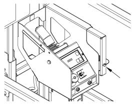
**Note:** For added protection, the platform control station can be secured to its mounting plate.
