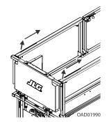
Rotate levers at the rear of the top platform rails and pull back to release the rails.
