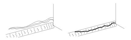
Figure 1. Parent Metal Crack
