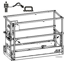
Figure 4. Lanyard Attach Points
