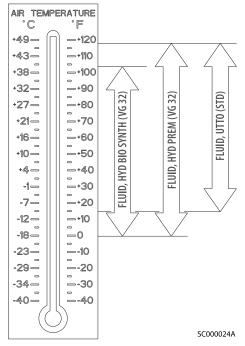
Figure 11. Hydraulic Oil Operating Temperature
