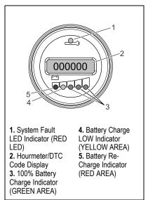
Also located on the MDI are Battery Discharge Indicators (BDI) (3, 4, 5). The three green LEDs indicate the level of charge (voltage) remaining in the batteries.
