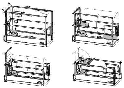
Figure 5. Rail-in-Rail Fold-Down Sequence
