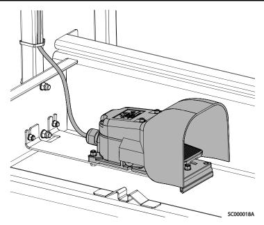
The footswitch serves as another enable switch in the function control circuit. It must be depressed in sequence with the platform control joystick trigger switch to enable operation of machine functions when using the platform controls. Power is removed from the platform controls when the footswitch is released.
