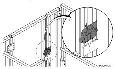
Figure 10. Magnetic Gate Latch Assembly
