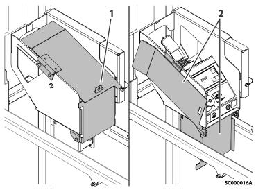
Figure 8. Platform Control Station
